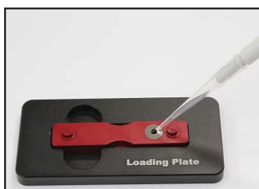
Pipette the Reference / Sample in turn.
